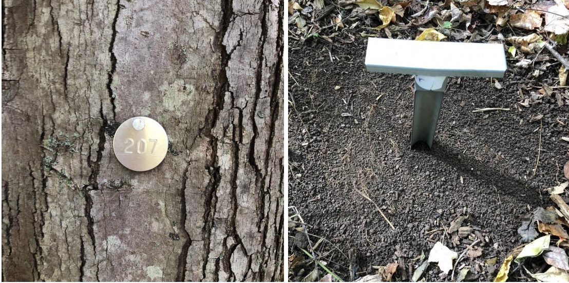
Figure A-2: (Left) Tree tag at breast height on a red maple in Plot C. (Right) Soil auger partially hammered into the ground before removal, measurement, and bagging of soil for bulk density calculation.
